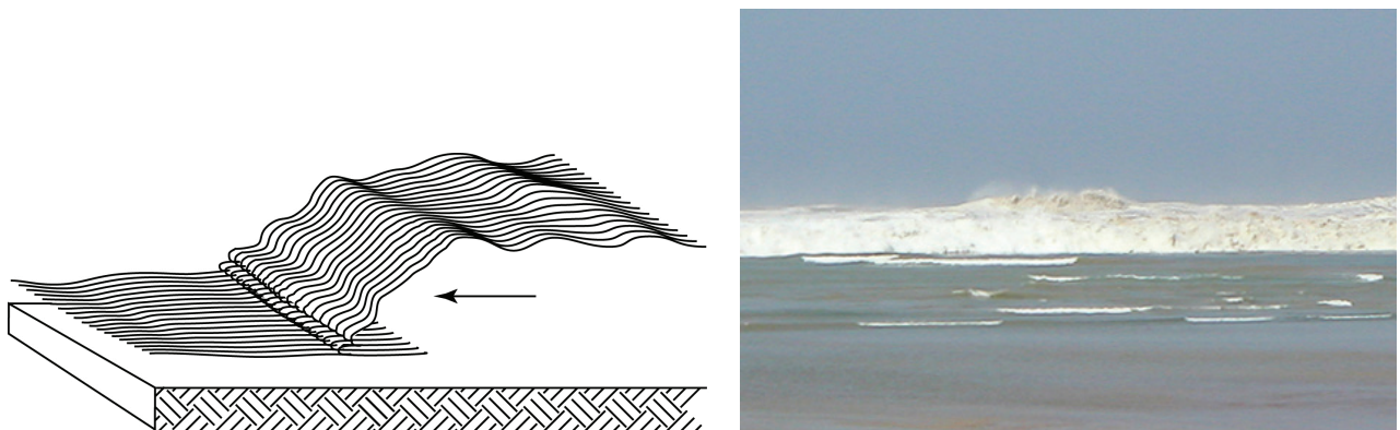
Figure 2-5 Sketch of a bore and photo of the 1983 Nihonkai-Chubu Tsunami showing the formation of a bore offshore (photo from Knill, 2004).
